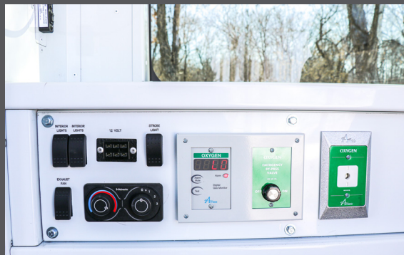
Rear Heat & Air Conditioning controls in rear compartment. Air is directed at the discretion of staff for ultimate comfort. Control panel includes power outlets and lighting controls.
