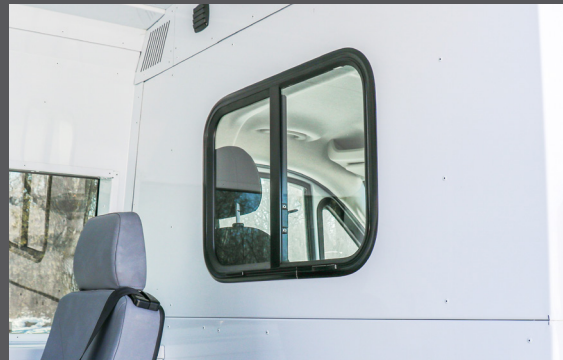
Cab divider available with or without window. Available with passthrough and sliding door options.
