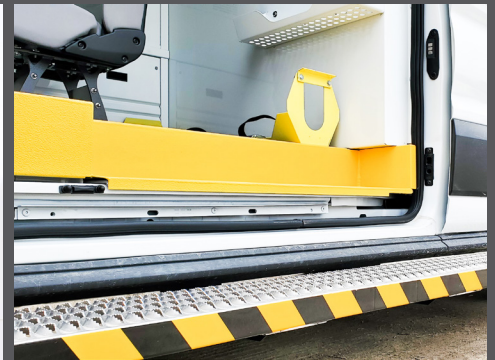
Serrated anti-slip running boards prevent ice and snow buildup
